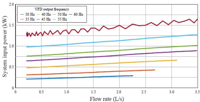
**Fig. 8** AWDS results with low zone in operation – System input power versus flow rate curves.
