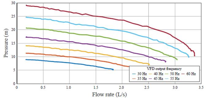
**Fig. 4.** AWDS results with low zone in operation – Pump head versus flow rate curves.
