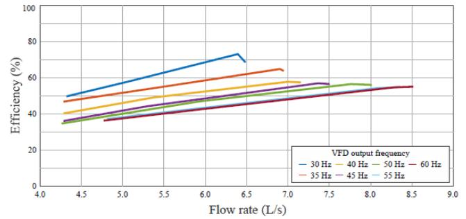
**Fig. 3.** PWDS results – VFD-motor-pump efficiency versus flow rate.
