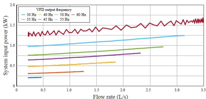
**Fig. 9** AWDS results with high zone in operation – System input power versus flow rate curves.
