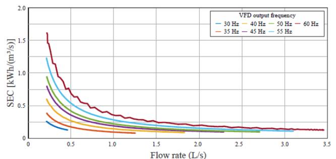
**Fig. 11** AWDS results with high zone in operation – SEC versus flow rate curves.
