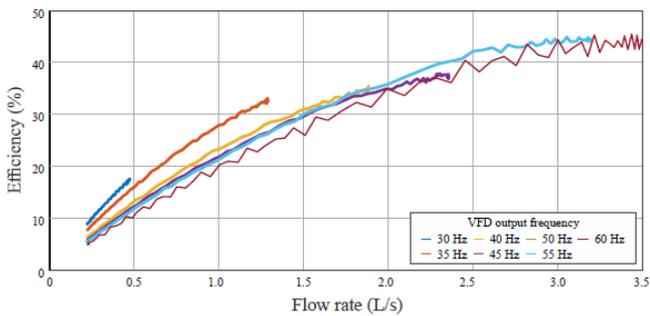
**Fig. 7** AWDS results with high zone in operation – VFD-motor-pump efficiency versus flow rate curves.
