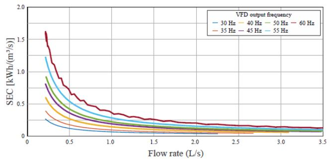
**Fig. 10** AWDS results with low zone in operation – SEC versus flow rate curves.
