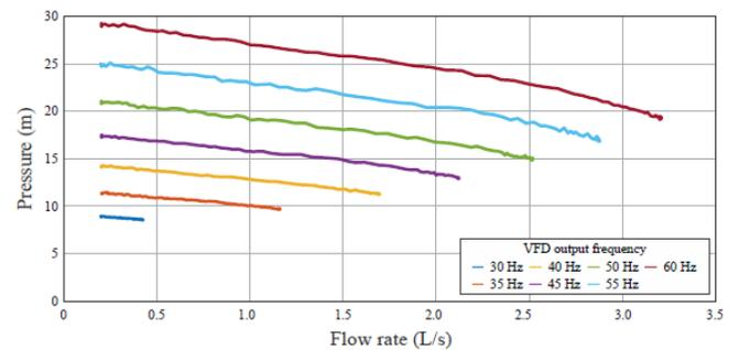
**Fig. 5.** AWDS results with high zone in operation – Pump head versus flow rate curves.
