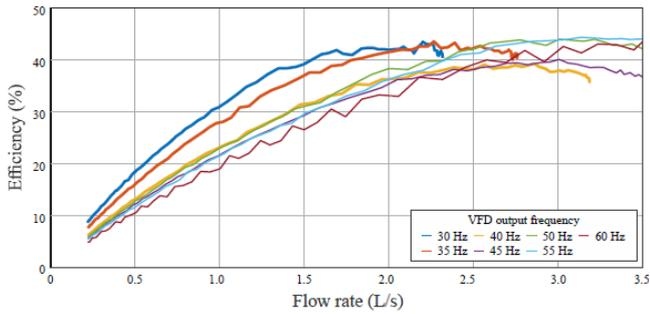
**Fig. 6** AWDS results with low zone in operation – VFD-motor-pump efficiency versus flow rate curves.
