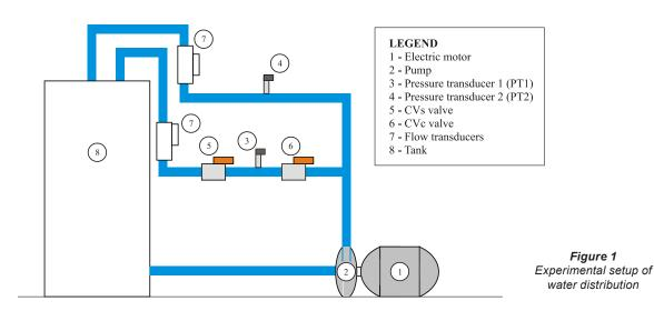
a demand variation. When CVs is closed, the flow decreases; consequently, the pressure upstream of the valve increases. The opening curve of the CVs curve was based on a profile of water consumption of a sector of the Metropolitan Region of Sao Paulo, Brazil.
