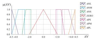
**Figure 5**Membership functions of the output linguistic variable  $\Delta V$
