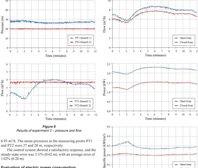
steady-state error was 3.11% (0.62 m), with an average error of 1.02% (0.20 m).
